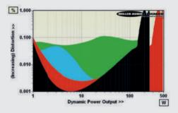
ABOVE: Dynamic power output versus distortion into 80hm (black trace), 40hm (red), 20hm (blue) and 10hm (green) speaker loads. Maximum current is 8.6A
