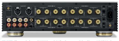
**ABOVE:** The one balanced XLR/three RCA line inputs are joined by an MM/MC phono input, subwoofer output and no fewer than 16x 4mm speaker cable posts. There are both A and B speaker banks with two amplifiers per 'channel' (one with optional highpass filter) for either bi-amping or bridging into two, single channel amps
